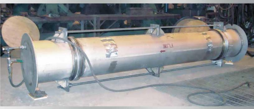
Hydrostatic testing of a universal expansion joint
